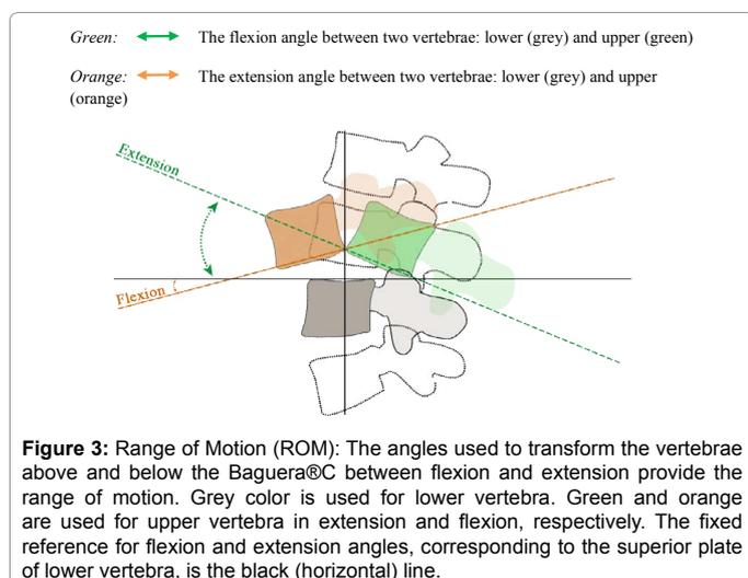
**Figure 3:** Range of Motion (ROM): The angles used to transform the vertebrae above and below the Baguera®C between flexion and extension provide the range of motion. Grey color is used for lower vertebra. Green and orange are used for upper vertebra in extension and flexion, respectively. The fixed reference for flexion and extension angles, corresponding to the superior plate of lower vertebra, is the black (horizontal) line.
